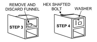
acceptor in place from the inside with the long hex-shafted bolt and washer provided.
